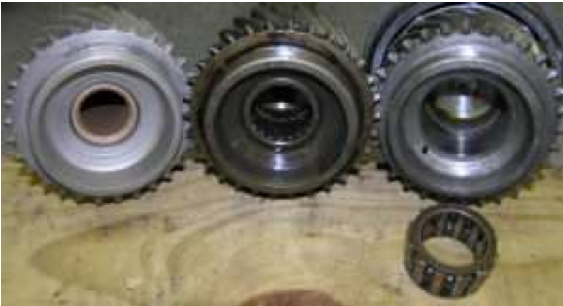
Step x – Remove mainshaft gears
