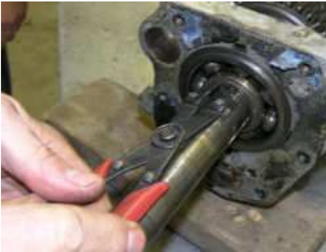
Step 7 – Remove the output shaft and countershaft gears
