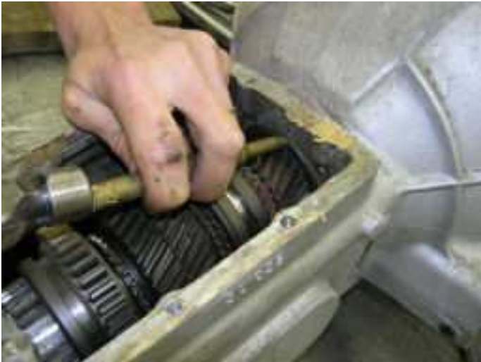
Step 10 – Remove the center bearing
