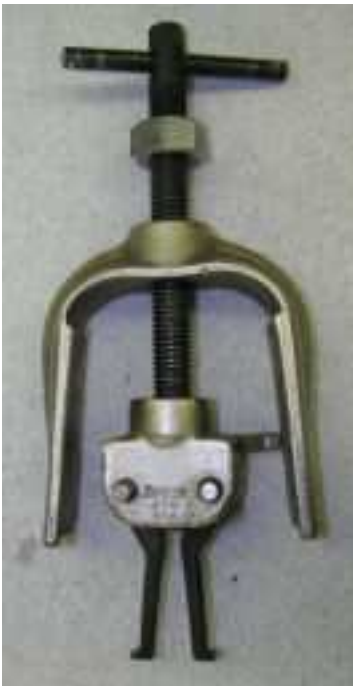
Step x – Remove input shaft bearing
