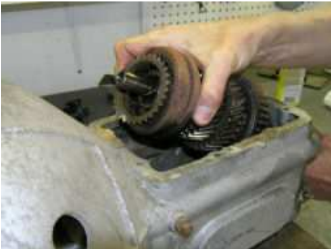
Step x – Remove Countershaft Bearings
