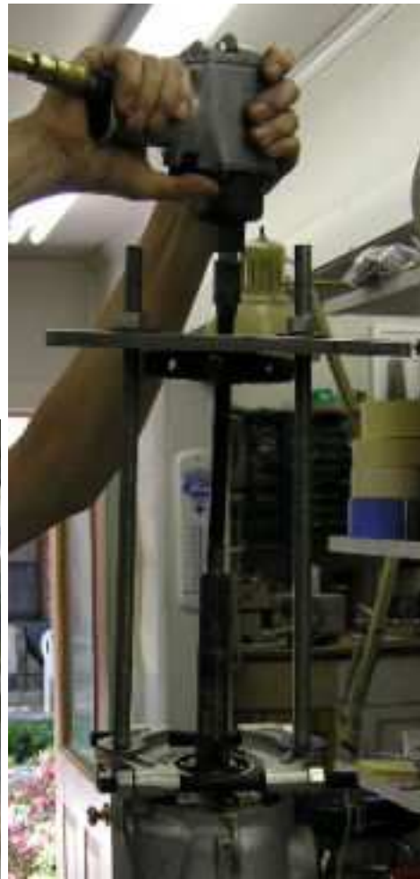
Step 7 – Remove the output shaft and countershaft gears
