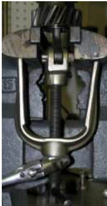
Step x – Remove input shaft bearing
